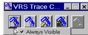
As mentioned earlier, with **VRS TraceControl** robot traces in the simulator can be controlled. A robot's trace is the trace left by the robot's active tool frame origin when it moves. Traces must be activated to be drawn, and they can be hidden or eliminated. The buttons for each of these options are the following:
